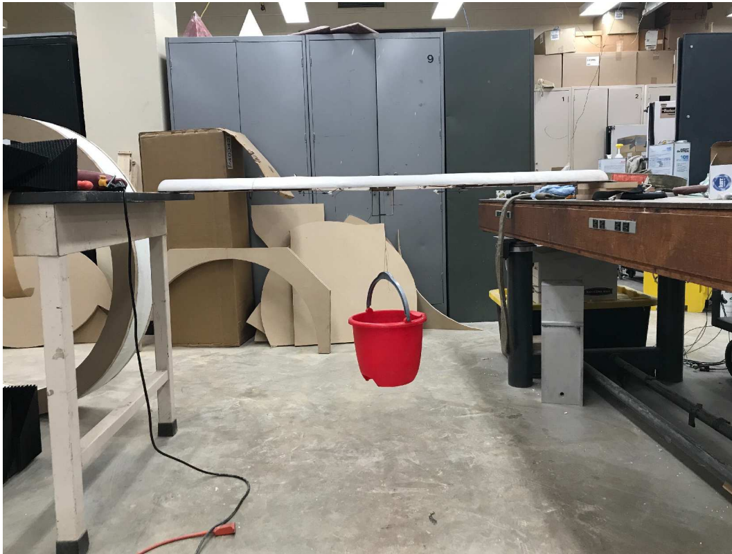
Figure 7.2 – Wing Loading Test
